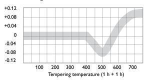
Note: The dimensional changes in hardening and tempering should be added.
