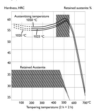
Above tempering curves are obtained after heat treatment of samples with a size of  $15 \times 15 \times 40$  mm, cooling in forced air. Lower hardness can be expected after heat treatment of tools and dies due to factors like actual tool size and heat treatment parameters.
