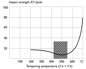
Tempering within the range  $425-550\,^{\circ}\text{C}$  is normally not recommended due to the reduction in toughness properties avoided.
