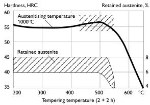
The tempering curves are obtained after heat treatment of samples with a size of  $15 \times 15 \times 40$  mm, cooling in forced air. Lower hardness can be expected after heat treatment of tools and dies due to factors like actual tool size and heat treatment parameters.
