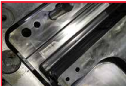
AISI D2 W.-Nr. 1.2379 uncoated with clear wear marks.
