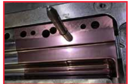
Caldie + Duplex-VARIANTIC 1000 with no visible wear. 1)
