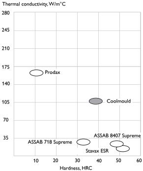
Note: Increasing alloying content gives a higher strength, but a lower thermal conductivity.
