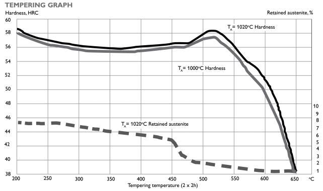
The tempering curves are obtained after heat treatment of samples with a size of  $15 \times 15 \times 40$ mm, cooling in forced air. Lower hardness can be expected after heat treatment of tools and dies due to factors like actual tool size and heat treatment parameters.
