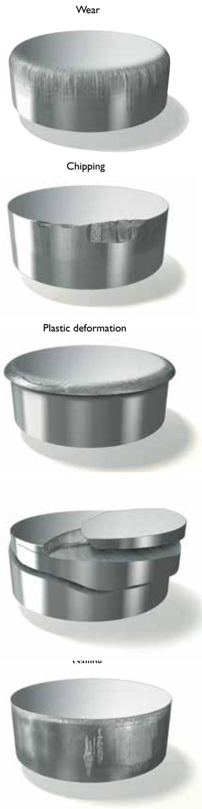
Figure 3. The most frequent failure mechanisms in cold work tooling.
