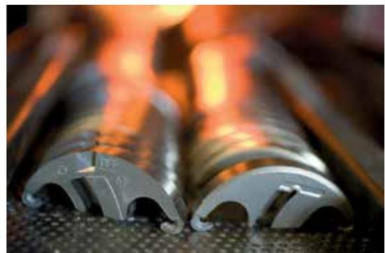
Sintering of powder compacted parts.
