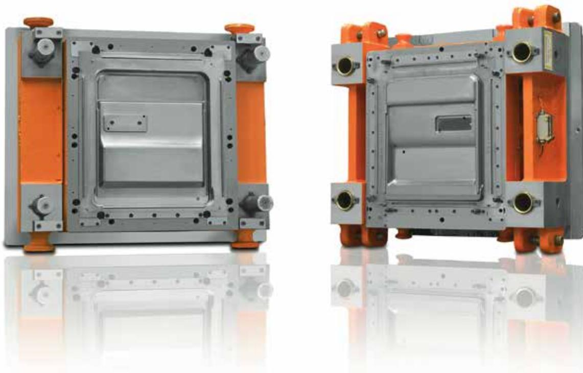
Tool of solid Vancron SuperClean for production of dishwashers.
