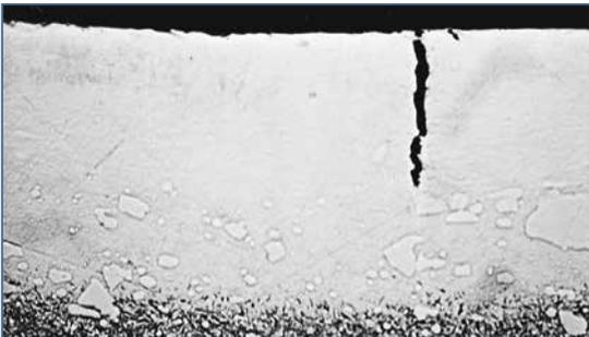
Photo 4. Surface of ASSAB XW-42 after rough spark EDM. The white layer is brittle and contains cracks.
