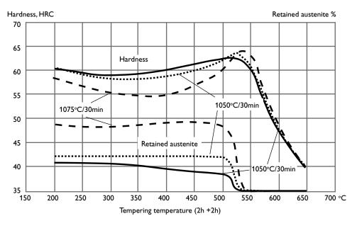
Above tempering curves are obtained after heat treatment of samples with a size of  $15 \times 15 \times 40$  mm, cooling in forced air. Lower hardness can be expected after heat treatment of tools and dies due to factors like actual tool size and heat treatment parameters.
