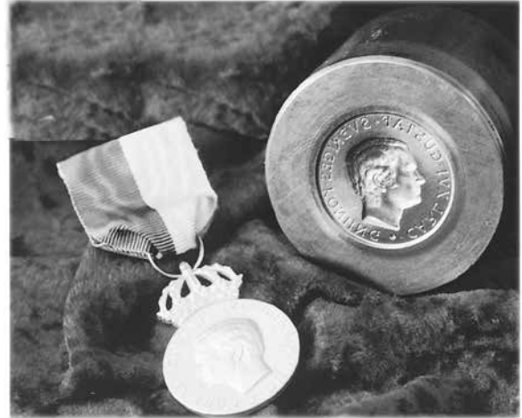
Cold work product where Calmax would be a good choice for the die.
