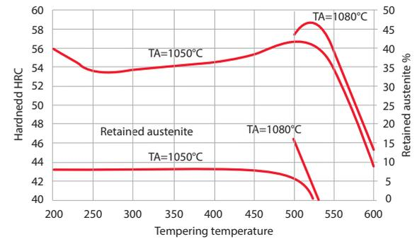
The tempering curve is obtained after heat treatment of samples with a size of 15 x 15 x 40 mm, cooling in a vacuum furnace.
