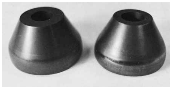
Vanadis 23 SuperClean (ASSAB PM 23 SuperClean) にPVD処理した冷間造管工具
