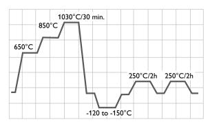
Subzero cooling is only required when demands on dimension stability during use are very high. Received hardness: 52-54 HRC.
